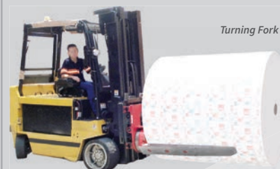
Clamp with Turning Forks
