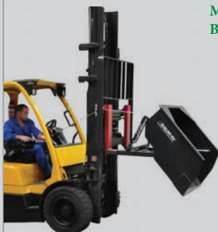
Tilting Paper Roll Clamp
