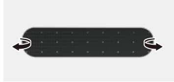
Double Diameter Herringbone Pads : Ideal for medium dense tissue, such as common facial and toweling grades. Flared end allows to reduce cutting of tissue at pad ends. Full radius edge allows paper to transition around pad without tearing.
